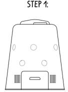
USING HOLE SAW, CUT HOLES IN THE COMPOST BIN, WITH THE SAME DIAMETER AS THE PVC PIPE.
