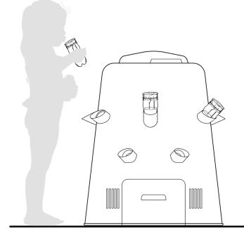
STEP 7: INSERT THE BOTTLE PROPAGATION UNIT INTO THE COMPOST BIN UNIT. THE FOAM INSIDE EACH PVC PIPE SHOULD SECURE THE BOTTLE FIRMLY. MONITOR THE SOIL TEMPERATURE IN EACH BOTTLE AND ADJUST THE DEPTH OF INSERTION AS NEEDED. ADD NEW COMPOST MATERIAL WHEN THE TEMPERATURE DROPS.
